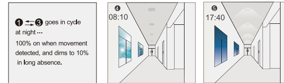
When the natural light level exceeds setpoint off to light, the light will turn off even if when the space is occupied. The light automatically turns on at 10% when natural light is insufficient (no motion).
