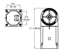
$\textbf{PMS}: \ \, \textbf{Secure} \ \, \textcircled{1} \ \, \textbf{and} \ \, \textcircled{2} \ \, \textbf{together and install the} \\ \text{fixture to the square pole.}$
