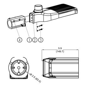
**WM**: Secure ① on the wall with 4 screws, then assemble ② to ③. Finally, install ② + ③ back to ① and secure.
