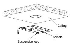
3. Connect the clip on the fixture to the spindle of the mounting plate to make sure the fixture will not slip and fall.connect the line voltage to the wires coming out from the fixture following the wiring diagram. Push the pressing plate into the suspension loop on the mounting plate.
