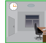
If with insufficient natural light switches off automatically after Semi bright brightness time standby period elapsed.
