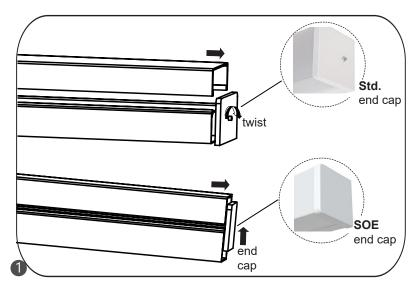
**Standard End Cap**: twist the knob to remove the end cap. **SOE End Cap**: Slide up to remove the end cap. Slide out the lens and unscrew the module plate inside.
