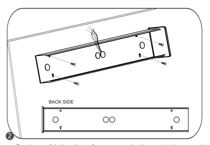
Punch any of the knockouts for power supply wires and make connection. Use (4) screws to install the fixture on surface.
